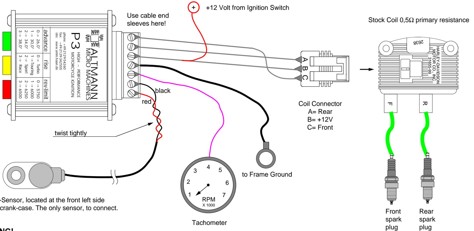
Crank-Sensor, located at the front left side of the crank-case. The only sensor, to connect.
